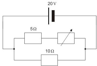
The resistance of the variable resistor is gradually increased from zero to  $5 \Omega$ .
