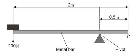
What weight is needed at position *P* to balance the bar?
