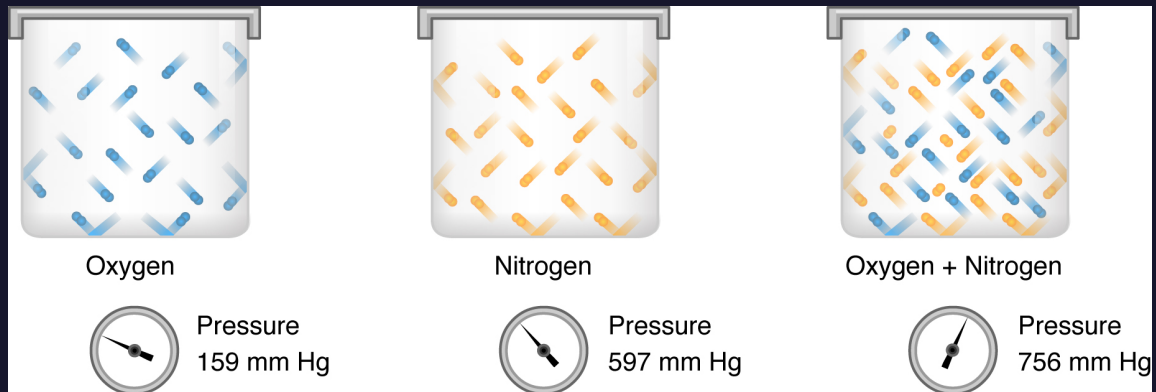
Figure 104: Partial pressure refers to the pressure that a gas exerts individually. When there is a mixture of gases, the total pressure is equal to the sum of the partial pressures of each gas present in the mixture. (Credit: openstax.org)
